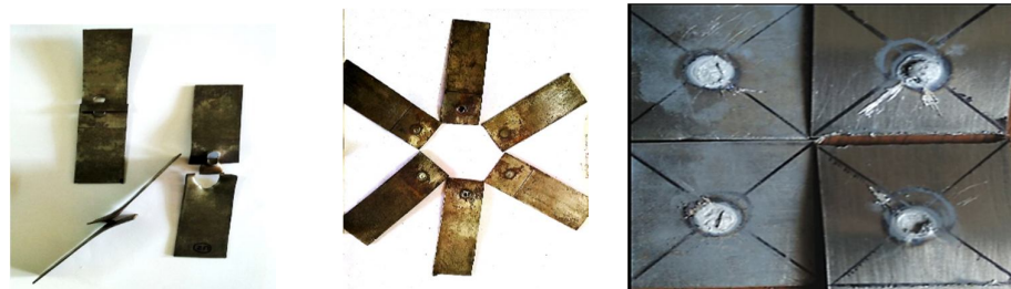
Fig. 7 (a) Pull out failure
